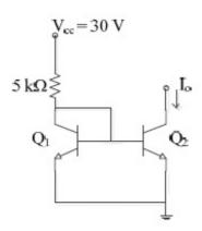
The current I<sub>o</sub> (in mA) is \_\_\_\_\_ (upto two decimal places)
